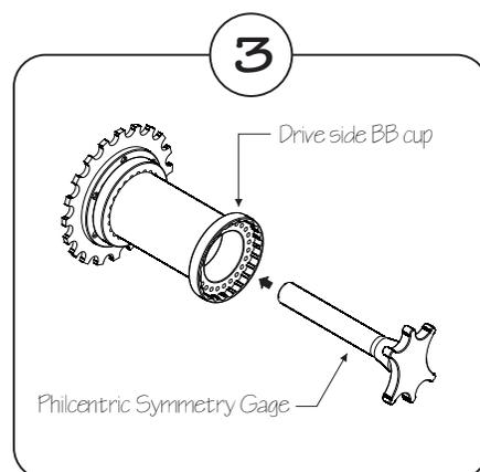
Insert the Philcentric Symmetry Gauge into the drive side BB cup. Ensure that the Symmetry Gauge is both centered and fully seated into the drive side BB cup.
