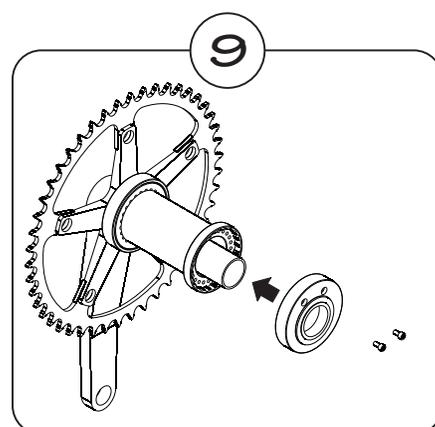
When chain tension is adequate, install the non-drive side Cup Cover.
