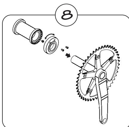
The crank must be removed followed by the Cup cover in order to make any adjustments to the chain tension. The Cup Cover can be rotated after it has been removed from the BB cup. Reinstall the Cup Cover, followed by the crank, and check the chain tension.
