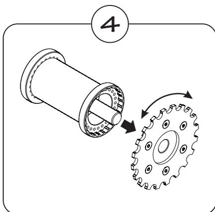
Remove the Cup Driver from the BB cup. Next, rotate the cup driver so that the alignment marks on the Symmetry Gauge and Cup Driver are as close as possible. Then, reinsert the cup driver into the bottom bracket cup.
