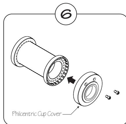
Install the drive side Cup Cover by lining up the dowel pin inside the Cup Cover with the notches inside the Bottom Bracket Cup. Press the two together by hand. Then install the screws to lock the two pieces together.
