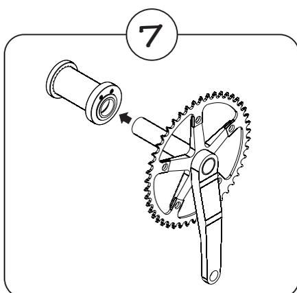
Install the drive side crank arm. Next, place the chain over the chainring and check the chain tension. If the chain tension is not adequate, the Cup Cover must be rotated to achieve optimum chain tension.
