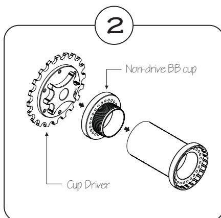
Apply blue Loctite to the non-drive side BB cup threads. Thread non-drive side BB cup into frame until the cup bottoms out against the frame. Then, loosen cup 1/4 turn.
