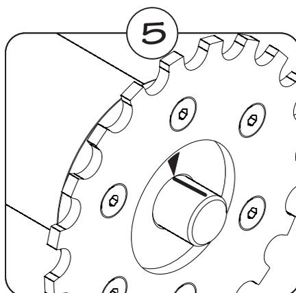
Turn the Cup Driver until the alignment marks on both the Cup Driver and Symmetry Gauge are lined up. It may be necessary to repeat step 4 in order to get the marks lined up. Once the marks are aligned, the cup should not be moved.
