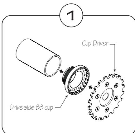
Clean the BB frame threads with alcohol. Apply blue Loctite to the drive side BB cup threads. Thread drive side BB cup into frame until the cup bottoms out against the frame.
